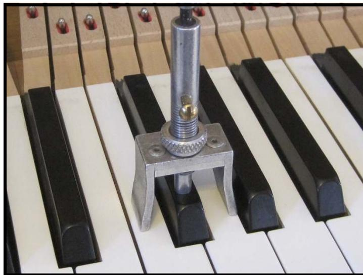
Sharp keys are leveled as well, as shown in the photo above. The approximate height of the top of the sharps over the top of the naturals is 1/2". Fine paper punchings are again used to make the sharps exactly level.
