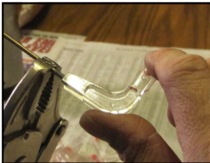
New plastic elbows being installed in a spinet.
